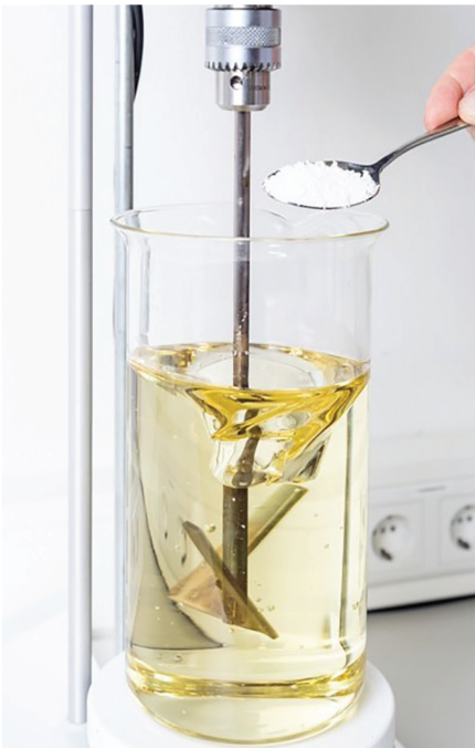
Addition of Ellamera polymer to warm oil
